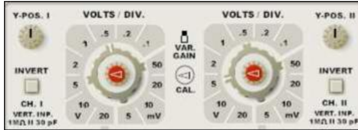
Figure 25: Vertical Controls of HM203-7 CRO
